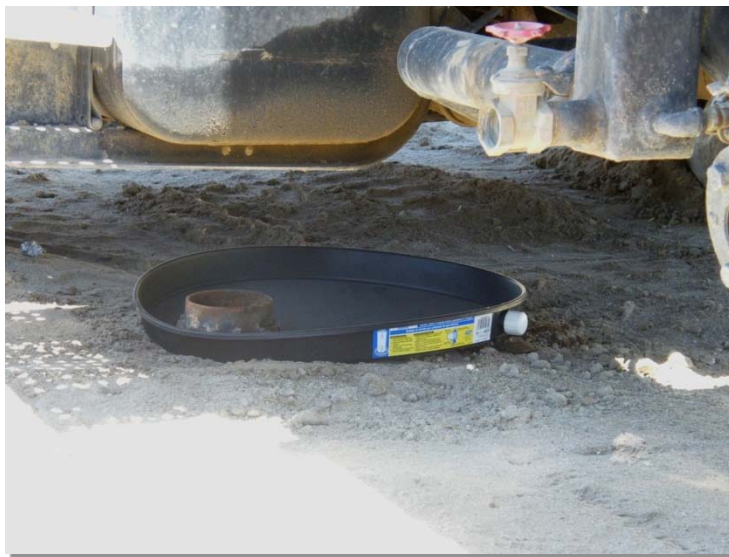
Photograph VF-1. Use drip pans to collect leaks from vehicles until repairs can be completed. Photo courtesy of Tom Gore.
