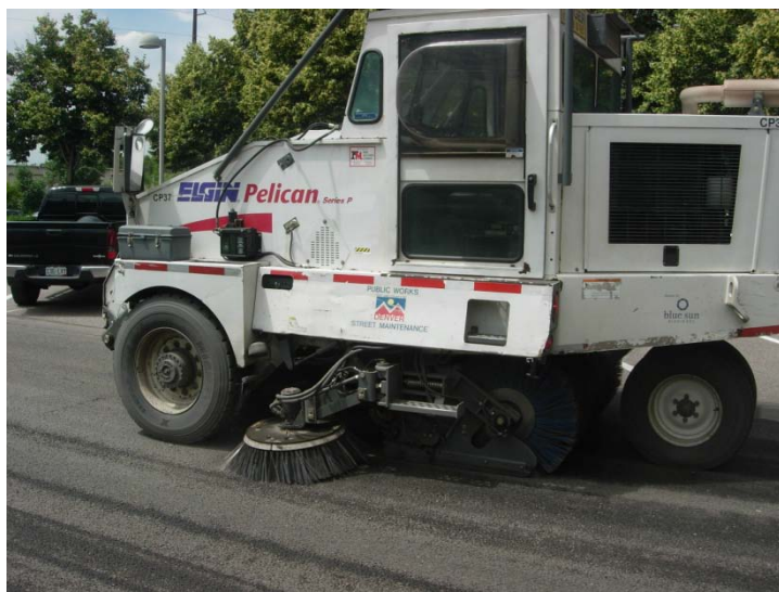
Photograph 6-4. This broom sweeper will only remove debris from the pavement surface. Broom sweepers are not designed to remove solids from the void space of a permeable pavement. Use a vacuum or regenerative air sweeper to help maintain or restore infiltration through the wearing course.
